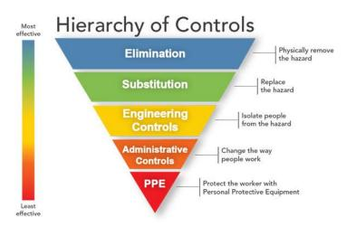
The following procedure(s) will be implemented for correcting identified hazards in the workplace:
